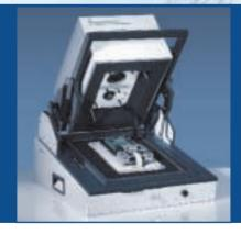
Our DUT fixtures can be upgraded to selfcontained small test stations, in which the mobile phone can be subjected to all tests – whether RF, acoustic, electrical or optical display inspection – in a one-stop test run.
