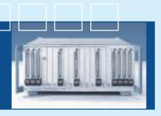
Based on cPCI/PXI, the TSVP system platform features outstanding flexibility. Up to 31 slots and the sophisticated bus concept allow practically any measurement, switching and control task to be implemented in a minimum of space.
